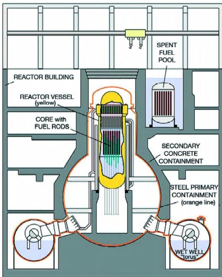
*Cross section drawing of a reactor unit with BWR reactor (Mark-1 reactor design)*
