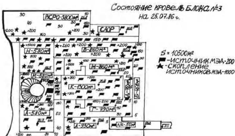
*On these roofs, adjacent to the destroyed Unit 4 reactor building, the fire-fighters got lethal radiation doses. (See explanations in the text)*
