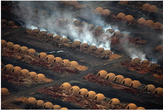
Figure 5. Beehive charcoal kilns in Brazil. Many trees must be burned, as the traditional process requires up to ten tons of hardwood to make one ton of wood charcoal.
