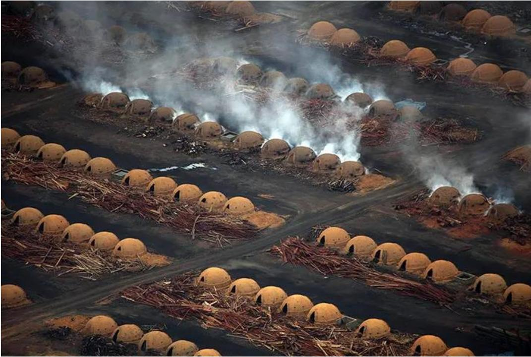
By weight, up to ~90% of the wood harvested is lost to the atmosphere as CO, CO<sub>2</sub>, smoke, and heat, so as much as ten tons of raw wood must be burned to produce a single ton of wood charcoal. [28][33] A few silicon producers claim to use dedicated “charcoal plantations,” but such plantations are limited in scope, so they can only supply a fraction of the overall demand for carbon in silicon production. [29-31]
