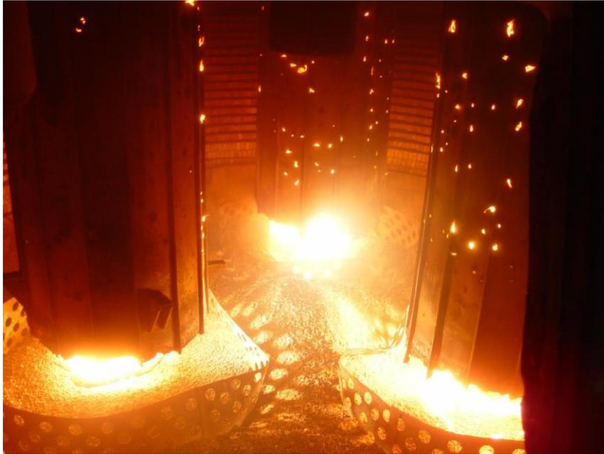
**Figure 2. In the silicon smelter, three 1-meter diameter carbon electrodes penetrate the surface of the charge of coal, coke, woodchips, and quartz rock. Each electrode is 10-20 meters tall.**
