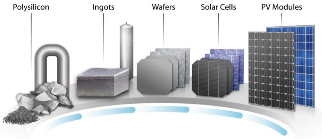
**Schematic of c-Si PV module supply chain**
