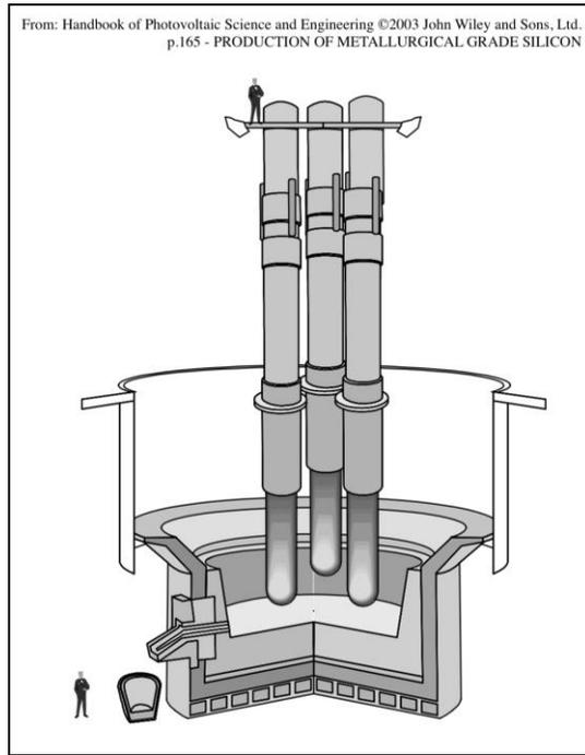
**Figure 1. Diagram of a silicon smelter showing the three giant carbon electrodes that provide arc temperatures > 3,000°F for smelting quartz into “metallurgical grade” silicon (mg-Si) using carbon as a reductant. ©2003 (John Wiley and Sons, Ltd.)**
