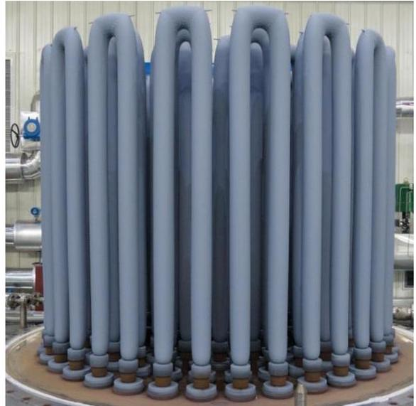
**Figure 5. Polysilicon rods grown in a CVD reactor. In this photo the CVD process is complete, the "bell jar" reactor dome has been removed, and the rods are ready for harvest.**
