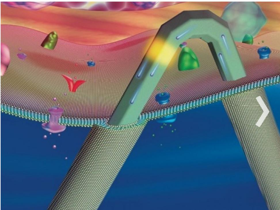
Hyman professor of chemistry Charles Lieber has created a transistor so small it can be used to penetrate cell membranes and probe their interiors, without disrupting function. The transistor (yellow) sits near the bend in a hairpin-shaped, lipid-coated silicon nanowire. Its scale is similar to that of intra-cellular structures such as organelles (pink and blue orbs) and actin filaments (pink strand).
